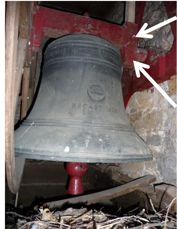
A plain stay on a metal headstock, just held in place with two bolts
